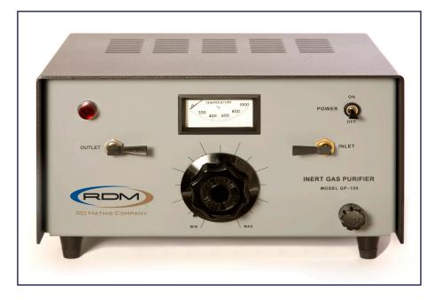
The GP-100 has been shown to purify 99.8% argon gas to 99.9991% purity as part of a worst case test. The principle impurity levels at flow rates of 1/4 liter/min. (0.53 cu. ft./hr.) were measured to be H<sub>2</sub> 0-2 p.p.m, N₂/C0-3 p.p.m., O₂-2 p.p.m., Ethane-1 p.p.m., other Hydrocarbons - no detection, and CO₂-1 p.p.m., with the limits of detectability set at 1p.p.m.\*
